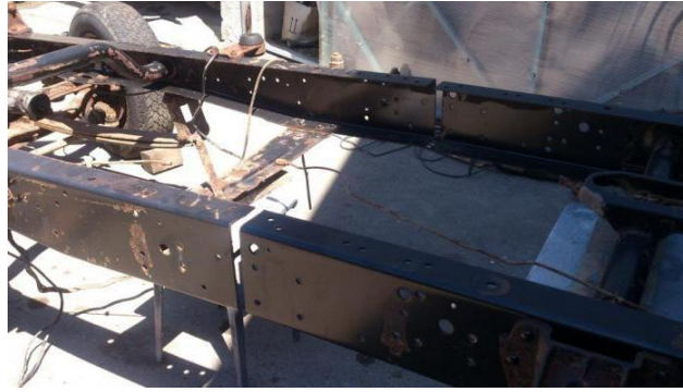
Fig. 3. Places, where the frame of the GAZelle NEXT car is cut
